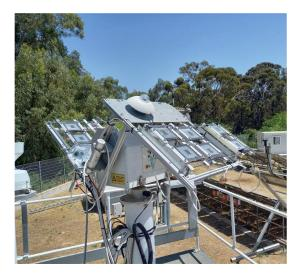
At all times, the degradation of modules tested outdoors is compared with the degradation of the identical control modules kept indoors in order to distinguish the effects of outdoor aging and intrinsic degradation. In most cases, the control modules present very good stability.
