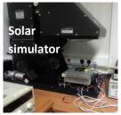
A Sol3A Class AAA steady-state solar simulator (Oriel, Newport) used to test solar cell performance under AM1.5 spectrum.
